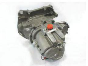
**3MO Performance** « ETCW » 2WD transmission has been designed by our R&D department to fit saloon or prototype car using transverse engine mounting. The gearbox specification meets a huge range of applications even for front or rear engine layout.
